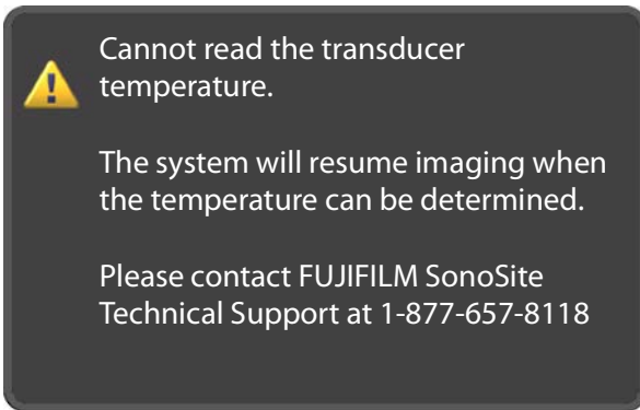
Figure 5-4 Transducer communication error message
