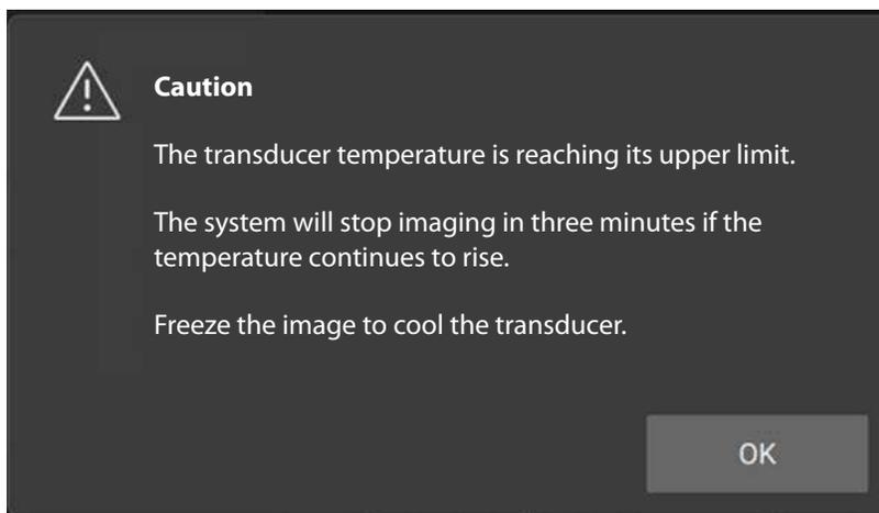
As indicated by the message in [Figure 13, "High temperature caution message" \[36\]](#), the system will stop imaging in three minutes if the scan head temperature stays above 43° C. Tap **OK** to dismiss the message, then either freeze the image to begin cooling the transducer or complete any remaining imaging within three minutes.
