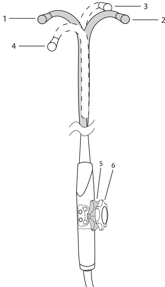
For orientation purposes, hold the transducer pointing away with control wheels up and the flexible shaft in a straight position.
