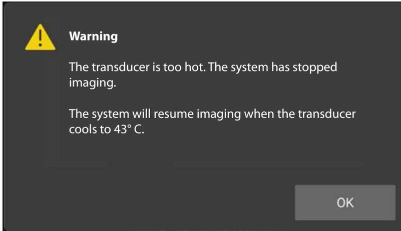
As indicated by the message in [Figure 14, “High temperature warning message” \[37\]](#), the system stops imaging if the scan head temperature remains above 43° C for more than three minutes or if it ever exceeds 45° C. Tap **OK** to dismiss the message and wait for the temperature to drop before resuming imaging.
