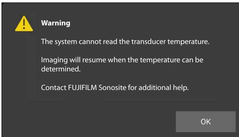
As indicated by the message in [Figure 15, “Transducer communication error message” \[37\]](#), the system stops imaging if the system cannot determine the scan head temperature. Tap **OK** to dismiss the message and contact FUJIFILM Sonosite or your local representative for assistance.
