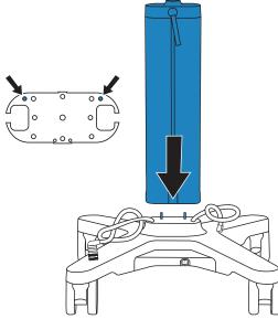
7. Use the provided 4 mm ball hex driver to secure the column to the stand with four M5 mm x 12 mm socket screws on the front, rear, and both sides.
