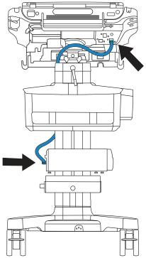
5. Connect the column power cable to the stand head by pushing it into place and screwing it into the connector. Tug gently to make sure it is secure.
