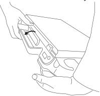
5. Connect the TTC connector to the system by placing the docking connector in the recess and turning the latch. Then fold the latch down.
