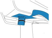
6. Slide an accessory mount assembly (double nut pad, mount, and two screws) into either the left or right channel of the stand column. You will install one on each side.
