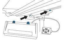
2. Insert screws, with insulating washers, through the screw holes in the stand head. Lift the TTC with your hand as you tighten the screws with the 2.5 mm hex wrench provided in the TTC installation kit.
