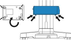
6. Insert two nut pads in the central rear column channel, and then slide them about 10% of the way up.
