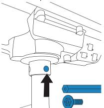
3. Use the same 5/32 hex key to tighten the two preinstalled screws in the collar.
