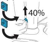
4. Slide another single nut pad up into the column and then secure the printer shelf with the 4mm hex key and two M5 hex screws.
