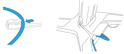
5. Connect the AC power cord to a hospital-grade AC mains outlet.
