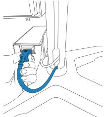
11. In both right and left channels, insert a cord catch and twist to lock it.
