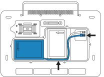
4. Attach the battery compartment cover using a Phillips screwdriver and the Phillips-head screws.
