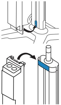
3. Slide the nut plate below the bottom mount and use the 4 mm hex key to tighten the M5 x 9 mm screw.
