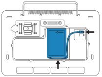
3. Place the other battery in the compartment as shown, then plug its cable into the connector. Make sure the cable is placed fully within the compartment.
