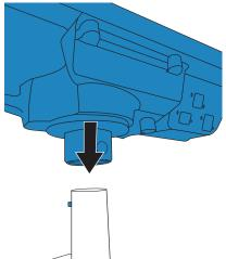
2. Use the security screw and 5/32 security hex key with the central hole to tighten the stand head to the post.
