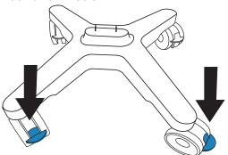
6. Locate the two mounting pins on the base and align them with the holes in the column.
