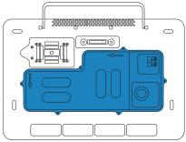
2. Place one of the batteries in the compartment as shown, then plug its cable into the connector. Make sure the cable is placed fully within the compartment.
