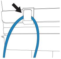
3. Install the AC cord hook on the same side as the power inlet.
