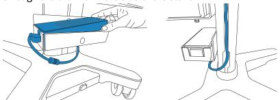
10. Plug the shorter cable coming up through the stand into the power supply.
