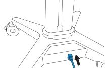
2. Run the AC power cord through the cord clip on the back of the storage tray. Alternatively, install the lower AC cord hook in the following steps. Both serve the same purpose. Wrap the cord if you need to wheel the system to an outlet.
