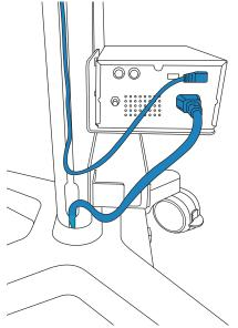
9. Place the power supply into the tray and then run the connected cable under the tray and up through the channel in the side of the stand.
