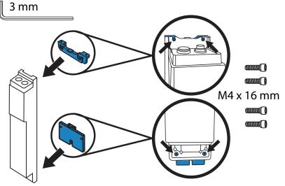
2. Slide the T of the bottom battery mount into the central channel on the front of the stand column. Raise the battery up until you can hook the top mount over the top edge of the stand column.
