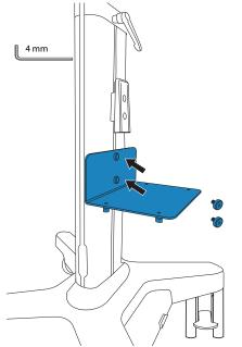
5. Set the printer on the shelf and then use the four thumb screws to secure it. The left thumbscrews use the holes at the rear edge of the printer. The right screws go through the rubber foot pads.
