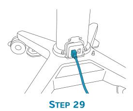
Connect the AC power cord to a hospital-grade AC mains outlet.
