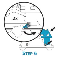
Turn the lid so the corrugated ramp supporting blocks are on the floor. Place the highest end near the platform and hook the corners of the lid over the metal corners of the platform.
