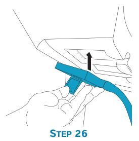
Press the latch handle up to secure the transducer connector to the stand head.
