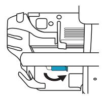
Connect the monitor cable to the engine. It is important to loop the cable as shown. Do not loop it in any other configuration.
