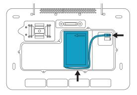
then plug its cable into the connector. Make sure the screwdriver and the Phillips-head screws. cable is placed fully within the compartment.
