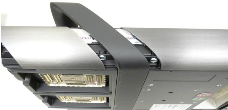
Figure 6.2 Side Extrusion Removal
