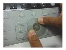
Figure 8-2: Removing the trackball retainer
