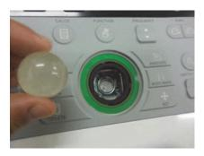
Figure 8-4: Trackball removed
