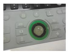
Figure 8-3: Trackball retainer removed
