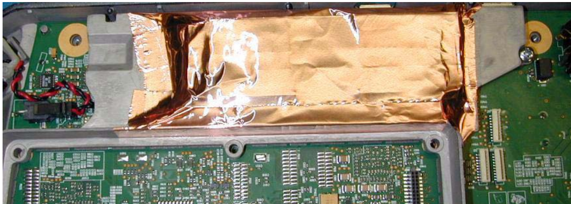
Figure 4.18 Copper Tape Installation - 3rd Strip
