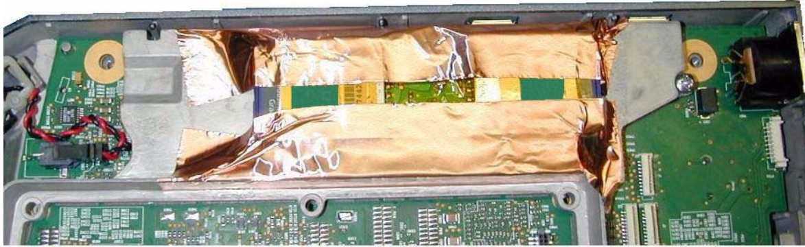
Figure 4.17 Copper Tape Installation - 2nd Strip
