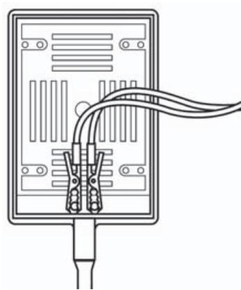
Figure 5-5 Transducer connector attachment
