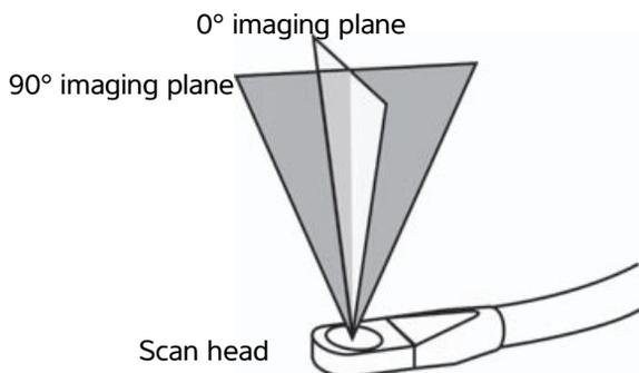
**Figure 2-1** Rotating to different imaging planes
