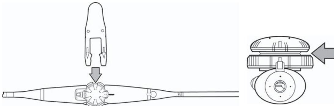
Figure 5-7 Insertion of the puncture test tool.
