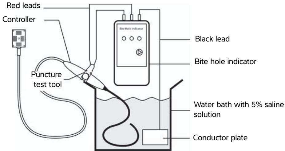
Figure 5-6 Endoscopic shaft test setup
