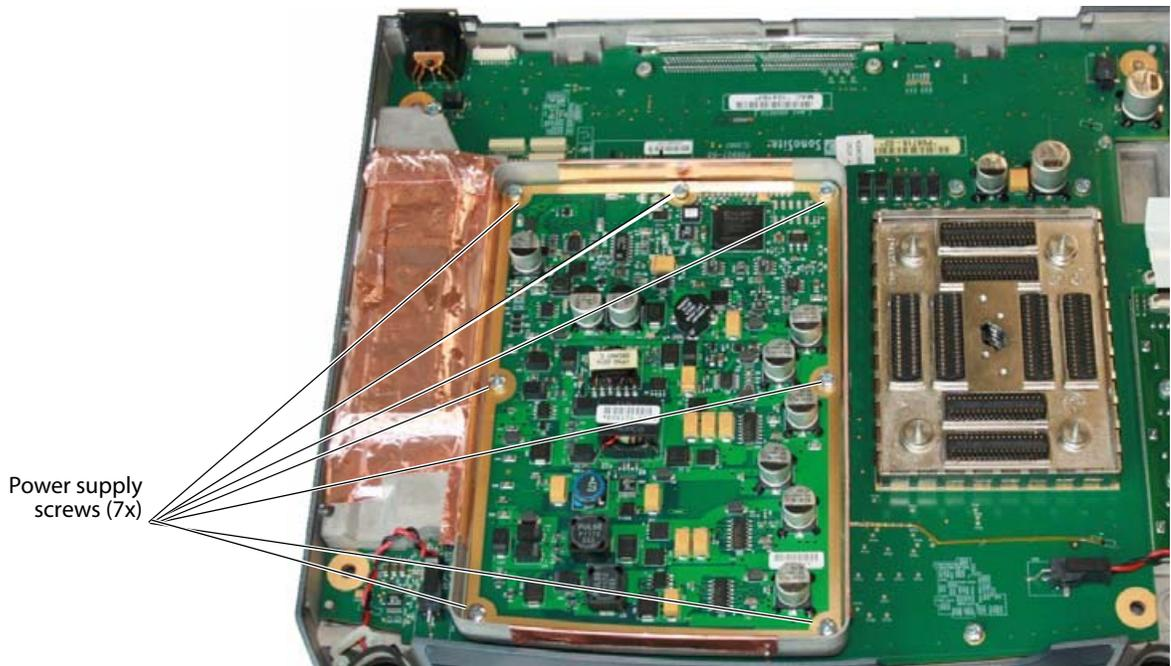
**Figure 4.10 Power Supply Screws**
