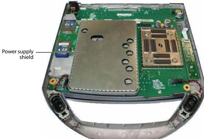
**Figure 4.9 Power Supply Shield**
