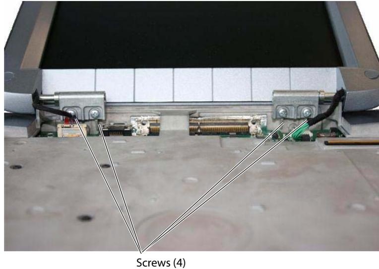
**Figure 4.6 Display Screws**
