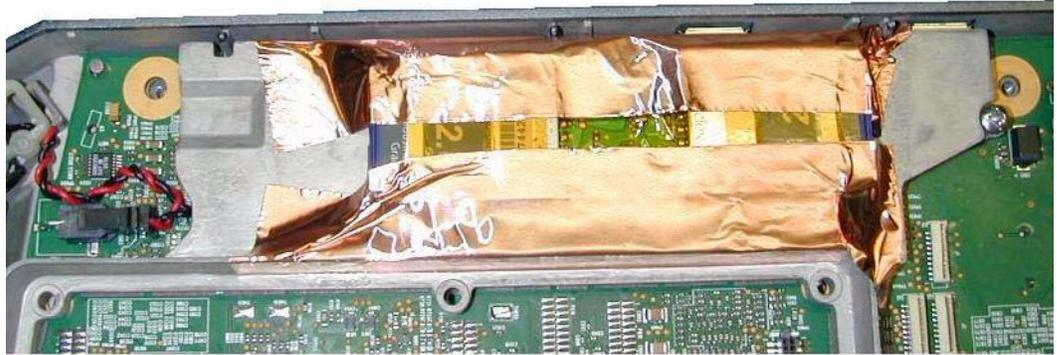
**Figure 4.15 Copper Tape Installation**
