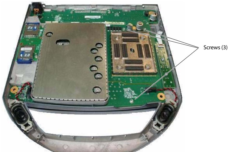
**Figure 4.20 Main PCBA Screws**
