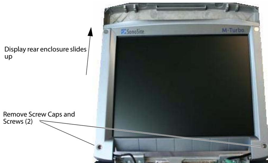
**Figure 4.5 Remove Display Back Enclosure**
