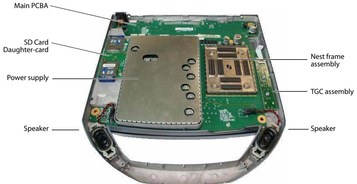
**Figure 4.7 System Components**
