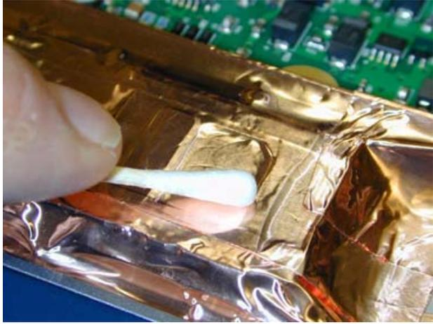
**Figure 4.17 Activating Copper Tape Adhesive**
