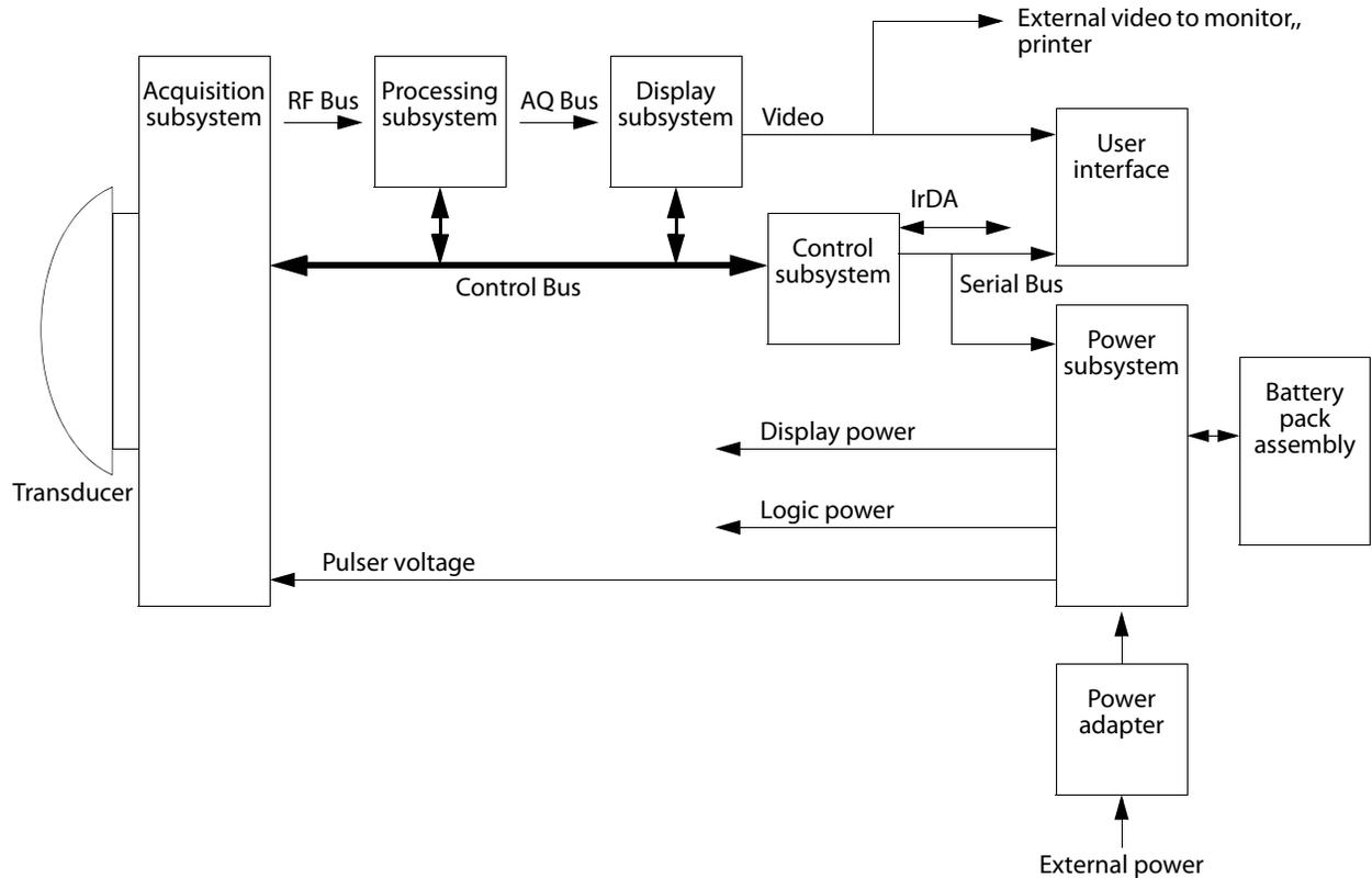
**Figure 2.1 SonoSite High-Resolution Ultrasound System (M-Turbo) Block Diagram**
