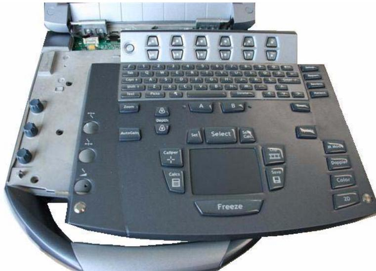
**Figure 4.3 Control Panel Removal**
