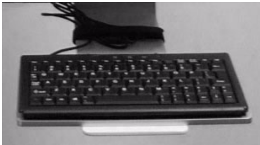
Figure 3 Keyboard with excess cable secured
