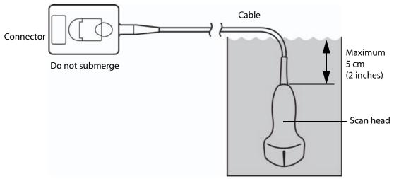
**10 Rinse** the transducer **3 separate times** using the following procedure:
