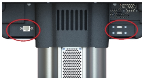
System connectors on back of the computer enclosure. Includes: Ethernet and USB connectors.
