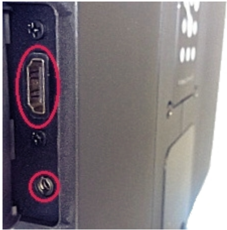
System connectors on back of the clinical display. Includes: HDMI and headphone jack connectors.
