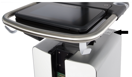
System enclosure with composite safety warning label location highlighted
