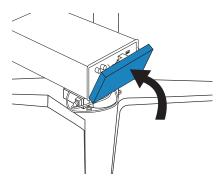
13. If you tilted the stand down to the floor, lift the stand back up onto the wheels.
