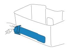
4. Slide the gel bottle holder down onto one of the mounting brackets on either side of the column.
