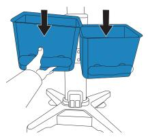
7. Install the two smaller bins on the front of the mounting bracket by sliding them over the mounts and then pressing down firmly to seat them.
