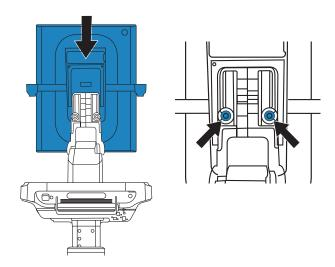
3. Tilt the clinical monitor back part way until you are able to feed the video cable up, and then connect the video cable to the rear of the clinical monitor. It is important to route the cable exactly as shown. Return the clinical monitor to vertical.
