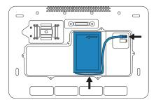
3. Place the other battery in the compartment as shown, then plug its cable into the connector. Align the arrow on the battery with the arrow in the compartment. Make sure both the cables are placed fully within the compartment.
