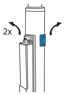
2. Push a cover plate in on both sides of the column.
