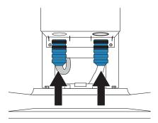
4. Screw the cable connectors clockwise to tighten.
