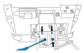
3. Connect the USB cable in the inner column to the USB port inside the stand head. Be certain that the USB cable is oriented correctly before pushing it in.
