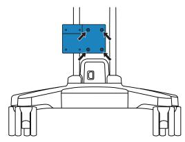
6. Slide the lip of the mounting box down onto the mounting bracket or stand, depending on which storage kit you have.
