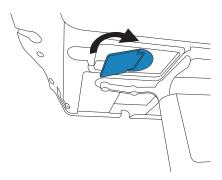
2. Flip the left and right latches up before placing the engine onto the platform.
