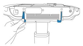
4. From the rear of the system, secure the connection between the engine and the transducer connector by rotating the latch counterclockwise and then pressing it up.
