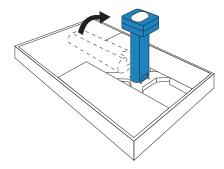
5. Use the bit driver with the 5 mm bit to tighten the four screws on the base of the column.
