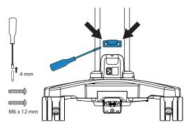
5. If you installed the four large storage bins, you must use the printer offset mounting bracket. Use the 4 mm bit driver and four M6 x 18 mm screws to install the printer mounting bracket to the stand.
