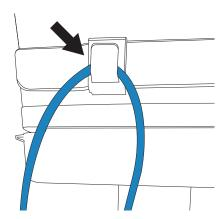
3. Connect the AC power cord to a hospital-grade AC mains outlet.
