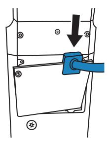
5. Attach the column cover to the stand by tightening the two M3 screws with the bit driver and the Phillips bit.
