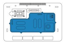
2. Place one of the batteries in the compartment as shown, then plug its cable into the connector. Align the arrow on the battery with the arrow in the compartment.
