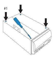
3. Remove the cover on the stand column with a pry tool.
