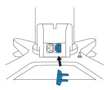
3. Install the cover at the bottom of the battery.
