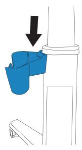
5. Slide the wipe holder down onto one of the mounting brackets on either side of the column.
