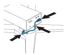
$9. \ \ \, \text{Connect the USB cable to the printer, and run the cable through the cable holder}.$
