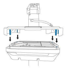
3. Use four M6  $\times$  12 mm screws and the 5 mm driver to secure the tray and monitor mount to the stand head. Insert screws from below the stand head into the monitor mount and tray. Do not use the rear mounting points.
