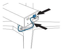
10. Plug the USB cable into the base of the stand.
