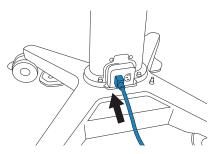
2. Run the AC power cord through the cord clip on the back of the storage tray. Wrap the cord if you need to wheel the system to an outlet.
