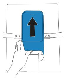
2. Carefully insert the blade of the tray and monitor mount into the rear of the clinical monitor and then use the Phillips driver to secure it with two M5 x 18 mm screws (screws are taped inside the cover).
