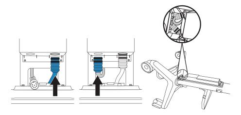
3. Push the cable connectors into place.
