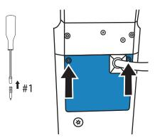
6. Connect the column power cable to the stand head by pushing it into place and screwing it into the connector. Tug gently to make sure it is secure.
