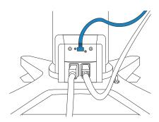
11. Install the cover over the USB connection.
