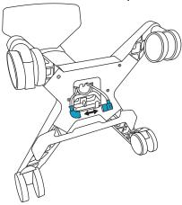
11. Attach the stand power connectors to the corresponding power receptacles on the PowerPark.
