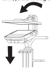
7. Lay the stand down on its front side, so that the longer legs are on the ground and the shorter legs face up.
