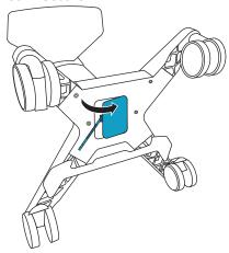
9. Reach through the access door into the base of the stand, and gently pull out the power connectors that are plugged together.
