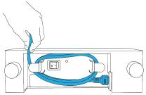
4. Position the dock on the floor against a wall, and connect the power cord to a hospital-grade AC mains outlet.
