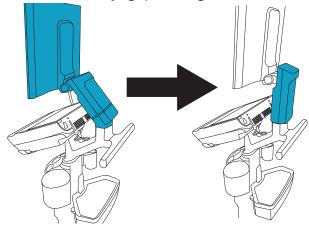
6. (Sonosite LX only) lower the stand column down to its shortest position, and rotate the clinical monitor down, parallel to the ground.
