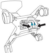
12. Set the PowerPark lip over the front edge of the stand base, aligning the four mounting holes on the PowerPark and stand.
