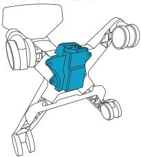
13. Use the magnetic driver with the 4 mm bit to attach the PowerPark to the stand using the four M5x35 mm screws.
