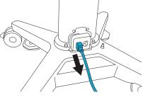
3. Press down the locking lever on each wheel.
