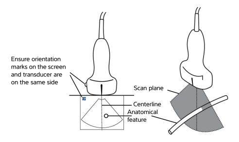
Figure 4-4 Relationship of the centerline graphic to the transducer and the ultrasound image.
