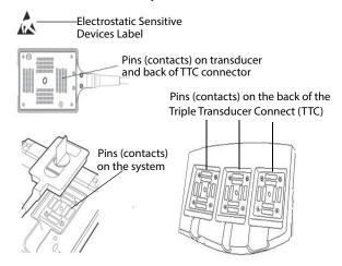
If the symbol is on a border surrounding multiple connectors, the symbol pertains to all connectors within the border.
