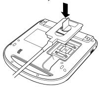
**2** Pull the transducer latch up, and rotate it clockwise. Align the transducer connector with the connector on the bottom of the system.
