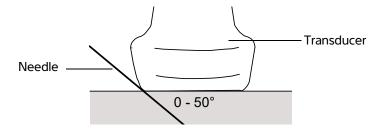
Figure 4-3 For best results, angle the needle only up to 50° from the transducer surface.
